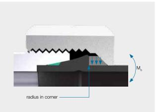
Transmission of dynamic loads by integrated clamping ring
