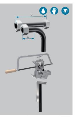
**2.2** Saw tube off at right angles. An angle tolerance of  $\pm$  1° is permissible. Do not use a rotary grinder or tube cutter.
