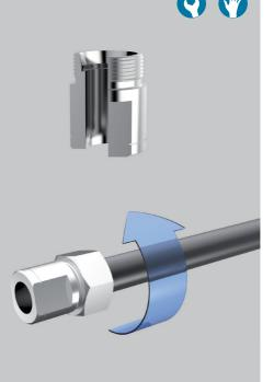
**4.1** Insert the tube end into the 24° taper as far as it will go and press on it. The tube must be held in as far as it will go during the entire assembly process in order to avoid faulty assembly.
