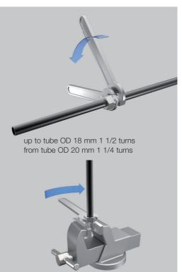
up to tube OD 18 mm 1 1/2 turns from tube OD 20 mm 1 1/4 turns
