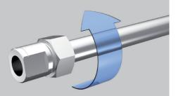
**4.3** Tighten union nut with approx. **1 1/4 turns** (min. 1 to max. 1 1/2 turns). This pushes the ES-4 cutting ring against the end face of the stud.
