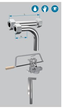
**2.2** Saw tube off at right angles. An angle tolerance of  $\pm$  1° is permissible. Do not use a rotary grinder or tube.
