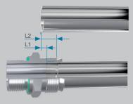
Height of the completely assembled VOSS*Form<sup>sQR</sup>*VA connection.
