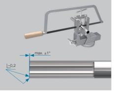
**2.3** Slightly deburr tube ends inside and outside. Clean the tube.
